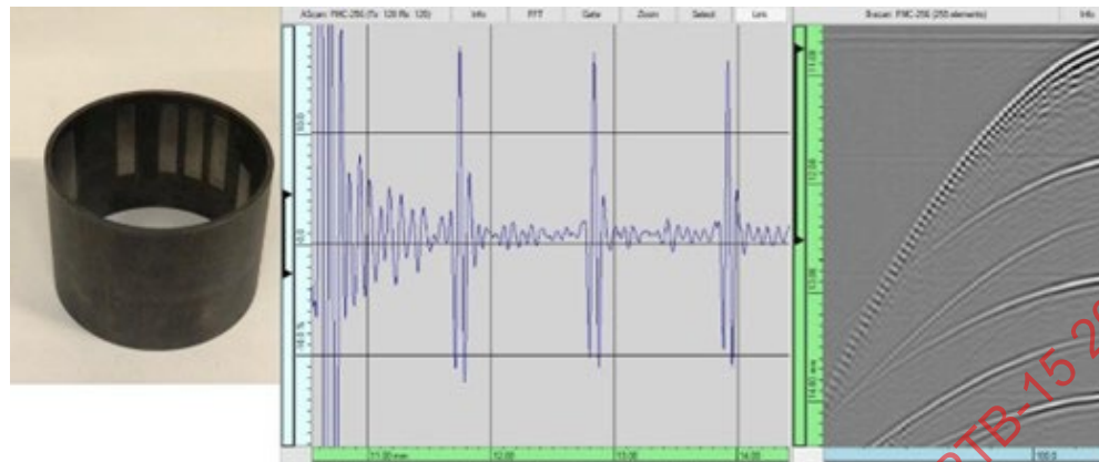
Figure 3-18: Sample, left with normal beam A scan response center. Note the phases remain consistent in each multiple.
