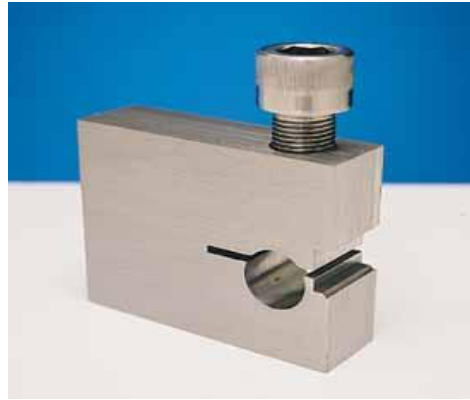
Figure 2 - Bolt-Loaded Compact Specimen
