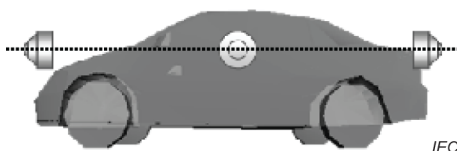
Figure A.2 – Camera mounting height
