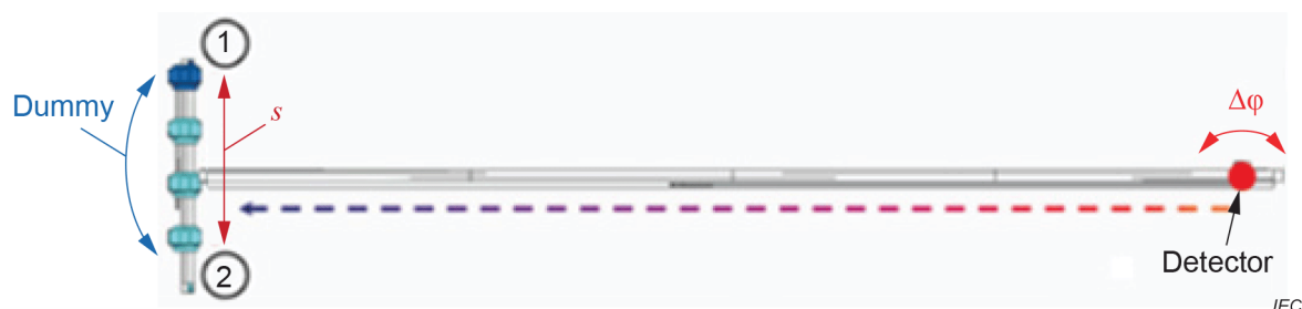
Figure 11 – Test setup for tangential movements (top view)
