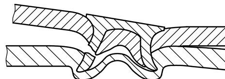
d) Rivet failure
