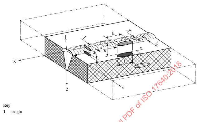
Figure 1 — Coordinate system for defining the location of discontinuities
