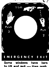
Figure A-1. The principal points to consider in gaining access to civil transport aircraft. Each aircraft must be examined individually to know how doors and windows may be most easily opened from outside.
