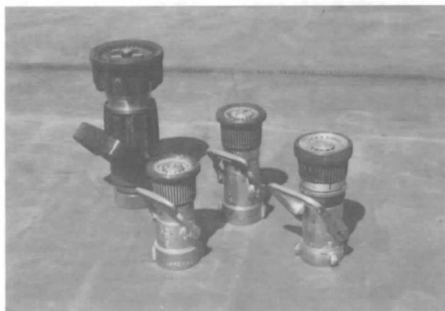
Figure 2-2.2 Photo shows a variety of typical spray nozzles currently used by structural fire departments. All have the feature of adjustable spray patterns from straight stream through a ninety-degree cone. Most fire chiefs agree that a nozzle setting of thirty degrees provides the best pattern for flammable liquid fire fighting with water or AFFF solutions.
