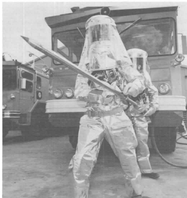
Figure 9-2.5 Aircraft Skin Penetrator Nozzle.
