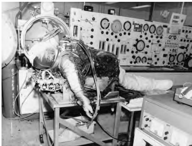
FIGURE D.2.6.7 Space Suit Destroyed in a Fire. No One Was in the Suit at the Time of the Fire. (Courtesy of NASA/Johnson Space Center.)
