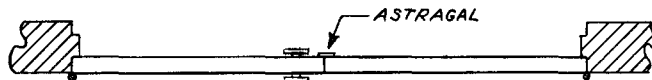
Figure A-21. Builders hardware (doors swinging in pairs with single point latch — flush mounted.)
