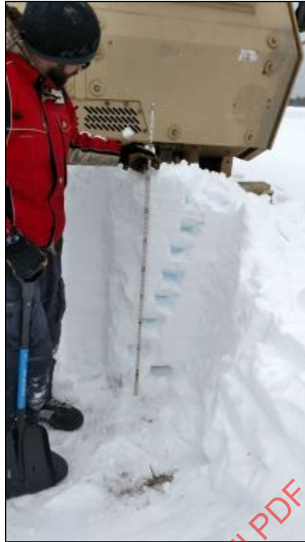
Figure A1 - Snow density measurements in snow pit (photo credit: Nevada Automotive Test Center)
